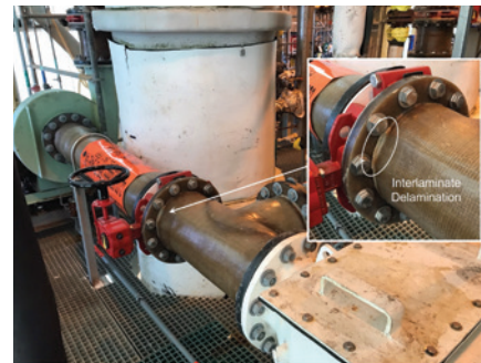
Figure 5. Flange hub radius interlaminar delamination.
