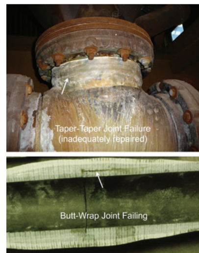
Figure 7. Secondary bond attack (adhesive and primary laminate).
