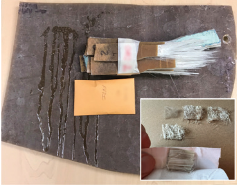
Figure 10. Remains of destructive test.
